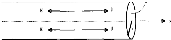
Fig. 1. A tube current pulse generating a uniformly charged disk and a uniform tube electric field.
