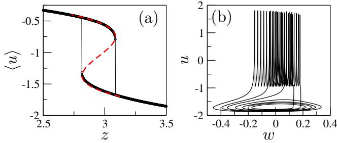
**Fig. 8.** (a) Dependence of  $\langle u \rangle$  on  $z$  for the fast subsystem Eqs. (6). The upper and lower branches correspond to periodic motion and stationary state, respectively. Red dashed curve shows approximating cubic parabola. (b) Phase portrait of system (5,6) demonstrates chaos in slow motion for  $J = -0.15$ ,  $\mu = 0.005$ . For better visualization only a short epoch with three bursts is depicted.
