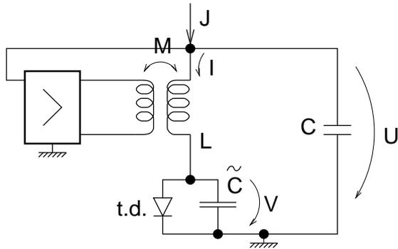
Fig. 1. Scheme of the KPR circuit driven by external current  $J$ .
